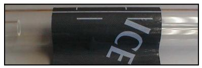
Figure 3-23: DMP-1 Dampening Material Wrapped Around Pipe
